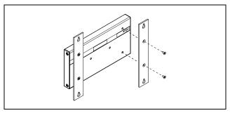
Figure 12. Compact FieldPoint Vertical Panel-Mount Kit with cFP-BP-4
